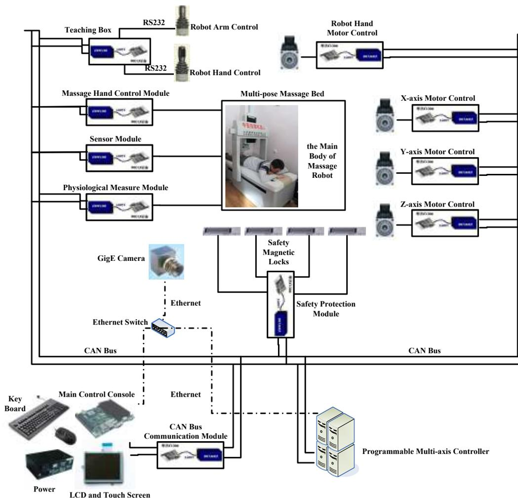
Figure 2. Logic diagram of physiotherapy service robot
